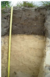
Plate 1. Typical profile of a two-year old reconstructed and rehabilitated sand dune. The topsoil exhibited a hard-setting zone below 0.05m depth and above the subsoil (tailings). Hard-setting refers to the strength of a soil tested under a specified moisture condition (moist and/or dry). In this profile the soil was hard below 0.05m, but the subsoil crumbled.
